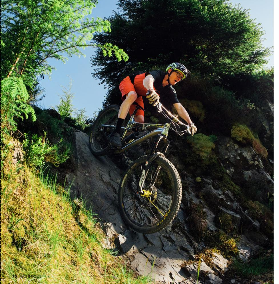
knowing where you are in the crank stroke will help you match the gear ratio to avoid having the cranks in the vertical at just the wrong time. More often than not in rocky terrain you need to drive a slightly larger gear to avoid having the cranks in the vertical too frequently.
