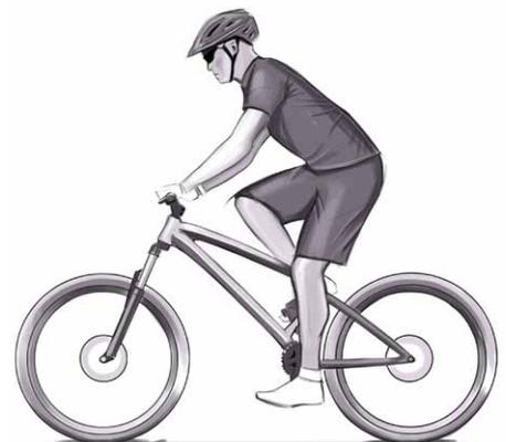
These geometry changes show a longer front triangle frame that situates the front wheel axle forward but keeps the handlebar in the same position thanks to a shorter stem. This is the key of the new **Forward Geometry** concept.
