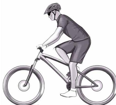
These geometry changes show a longer front triangle frame that situates the front wheel axel forward but keeps the handlebar in the same position thanks to a shorter stem. This is the key of the new **Forward Geometry** concept.
